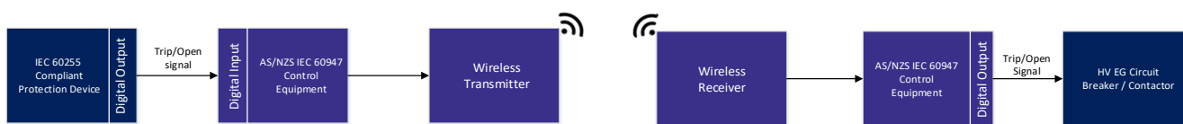
Figure 1: Typical Wireless Protection Trip Scheme
